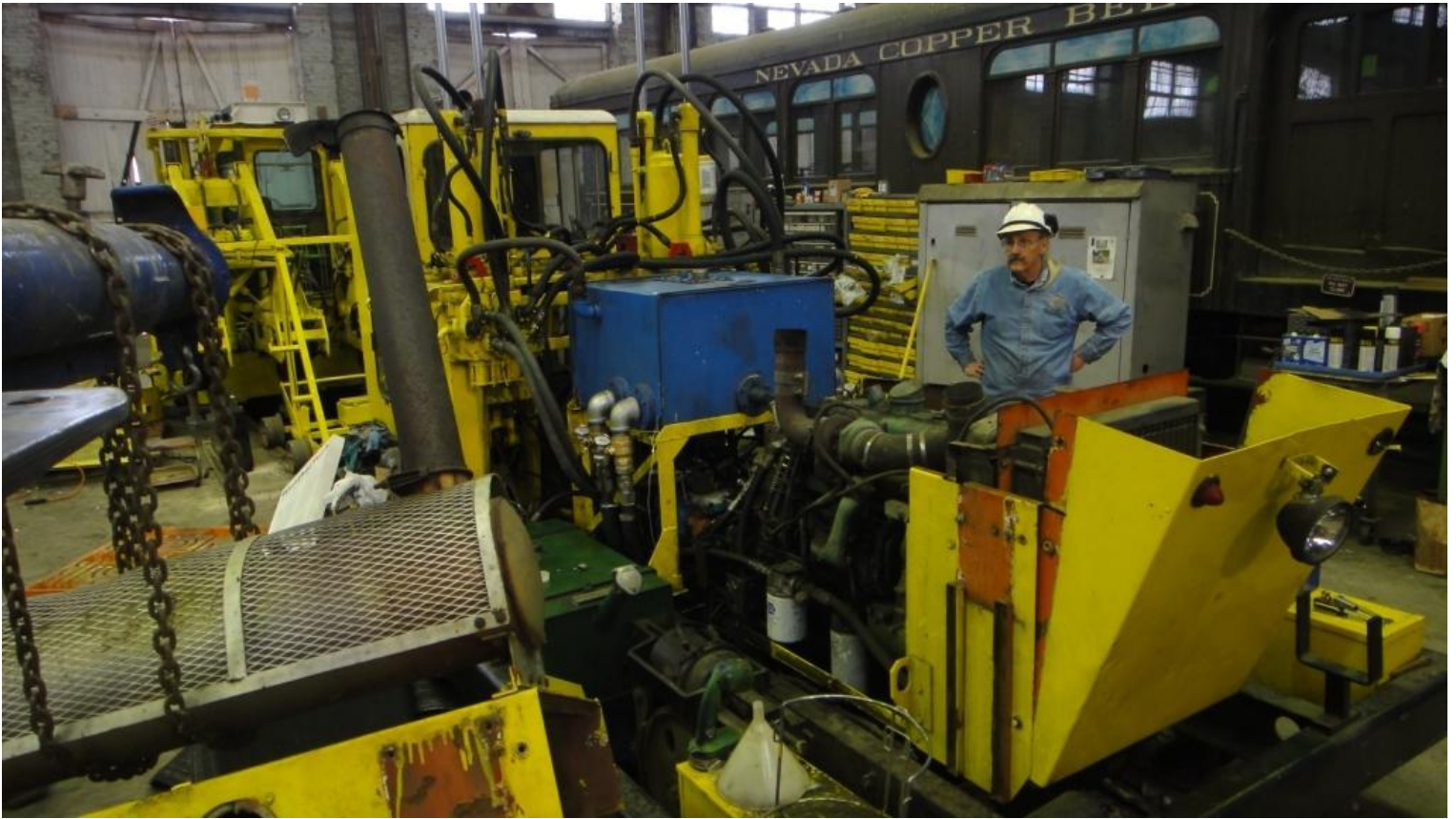
Fred awaits the shroud, muffler and smokestack (which is hanging by a chain from the stinger on the forklift to the left) for re-installation on the tie-shear.
