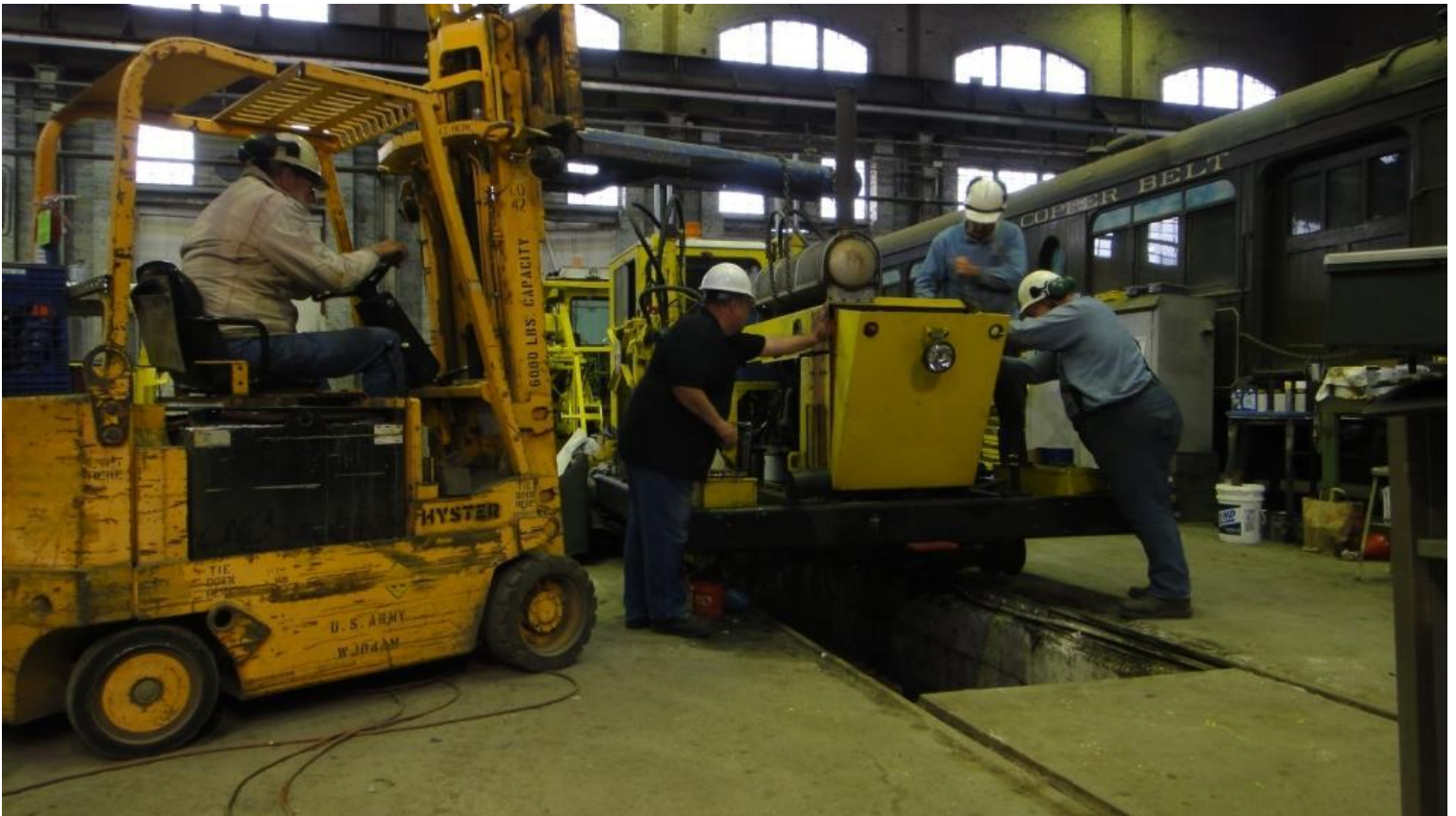
Alan on the forklift while Steve H., Fred, and Frank get the shroud and muffler into place.
